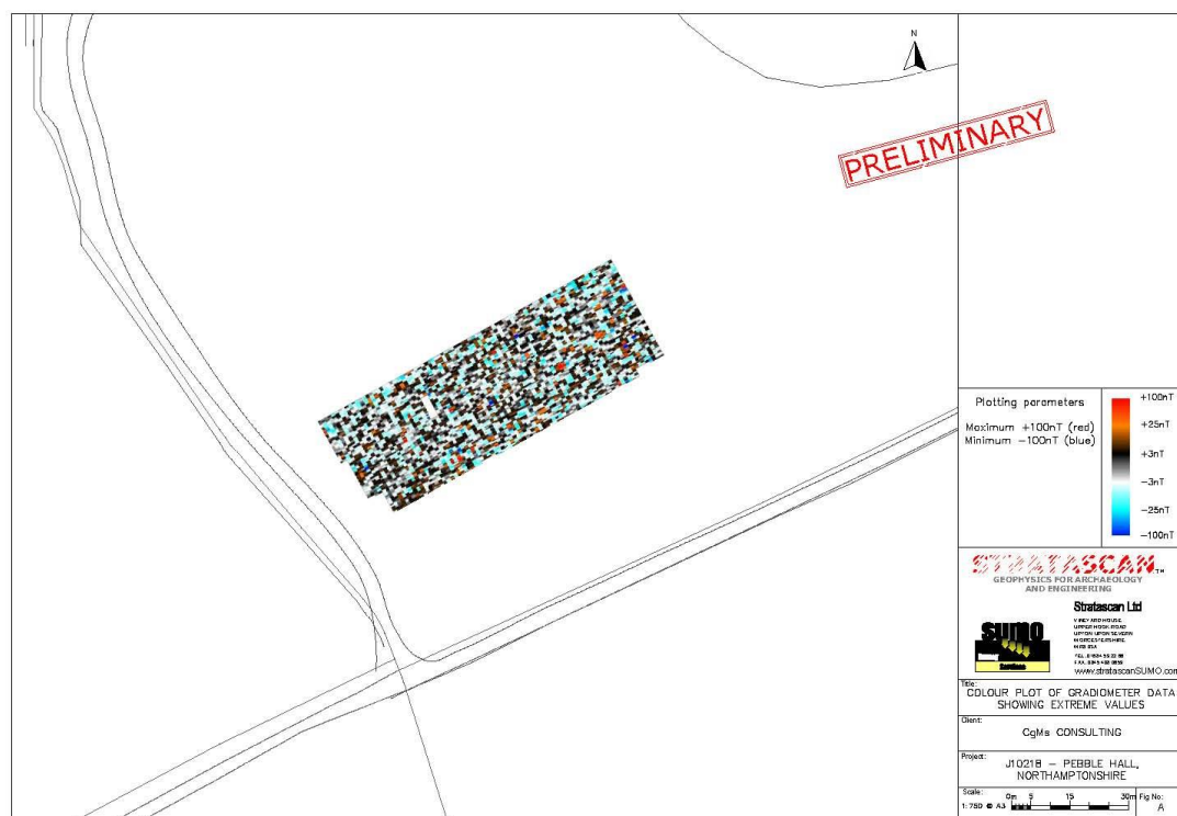
Fig 2 Sample area showing the masking effect of green waste at Pebble Hall
