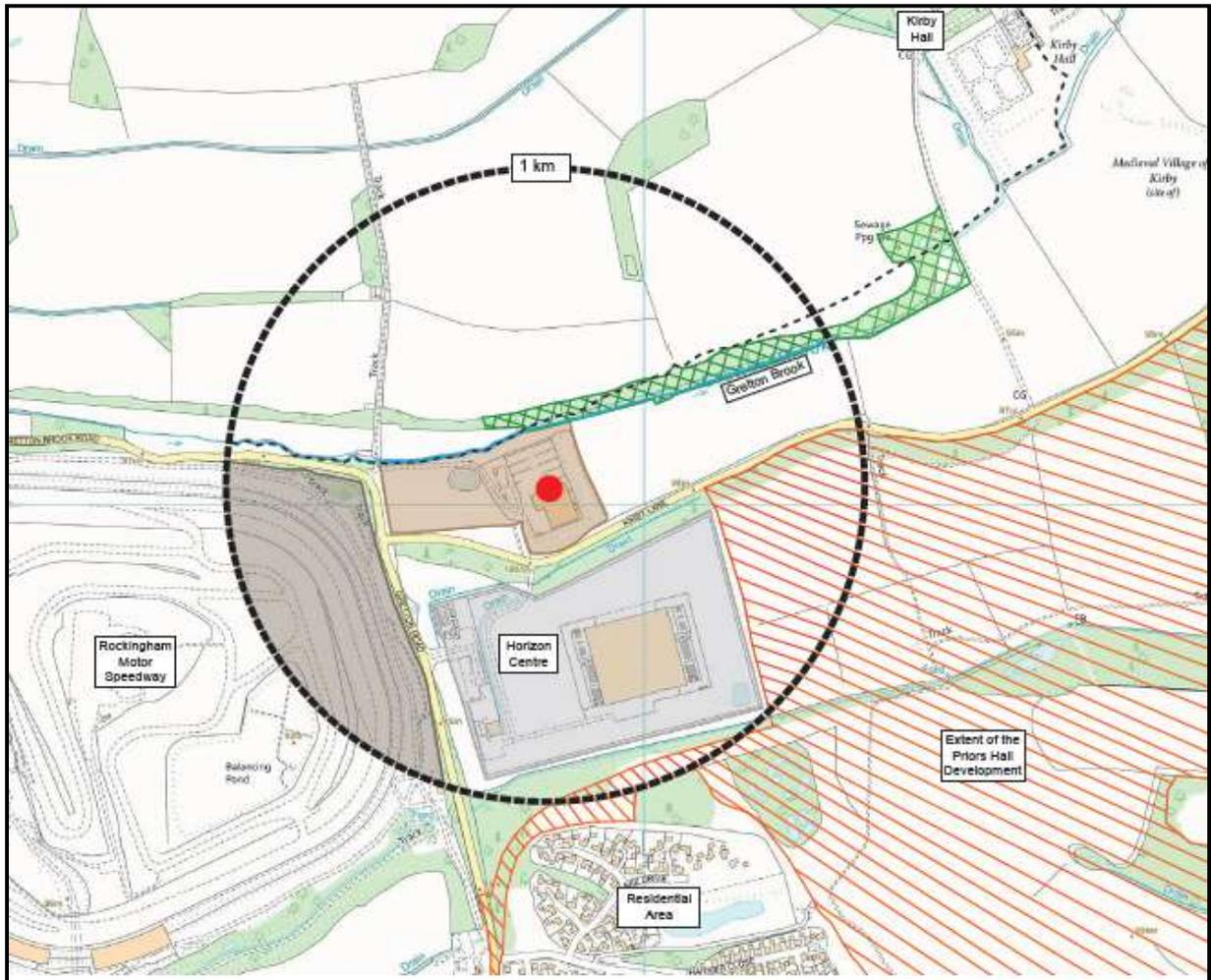
The ADMS 5.2 dispersion model has been used to make predictions of ground-level concentrations of odours occurring due to emissions from the facility.
