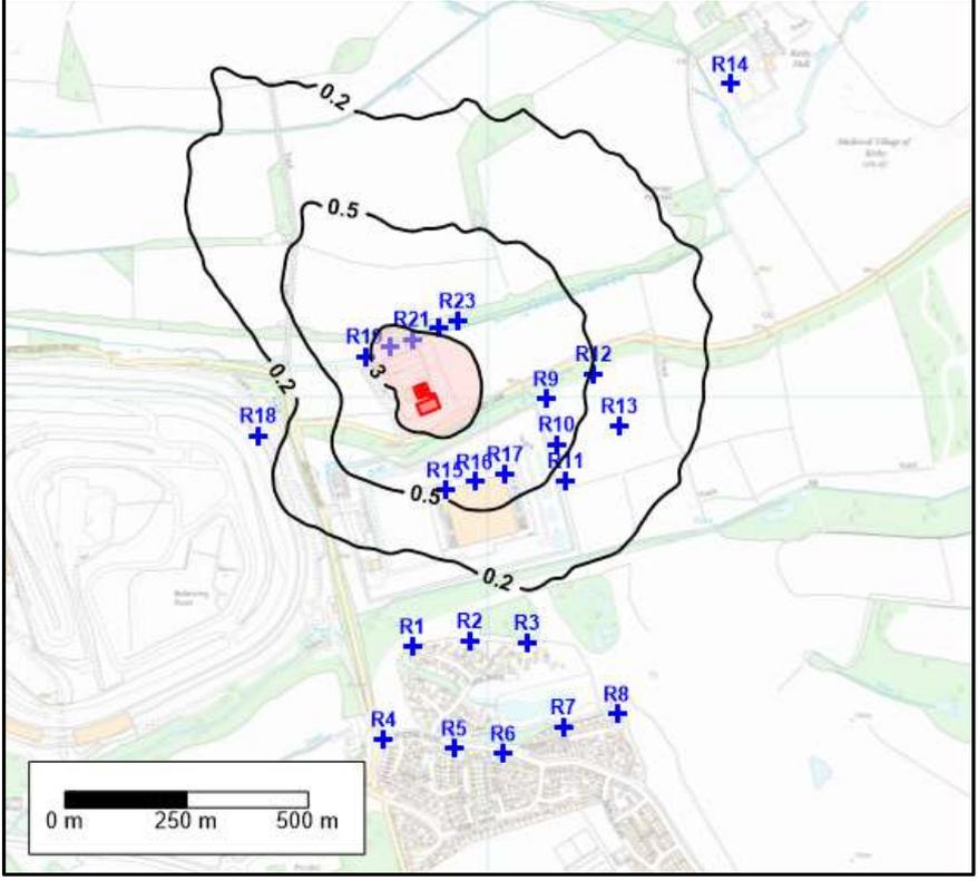
**Figure 5.4 ADMS 5.2 Predicted 98<sup>th</sup> Percentile of Hourly Average Odour Concentration, 2018 Meteorological Data (OU<sub>e</sub> m<sup>-3</sup>)**
