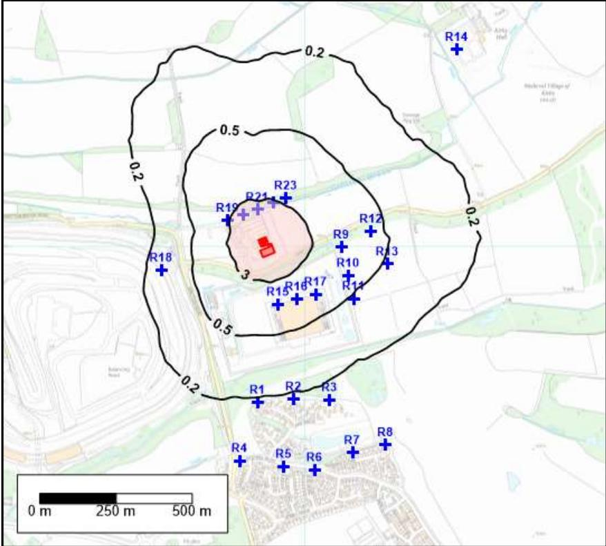
Figure 5.3 ADMS 5.2 Predicted 98<sup>th</sup> Percentile of Hourly Average Odour Concentration, 2017 Meteorological Data ( $OU_e m^{-3}$ )
