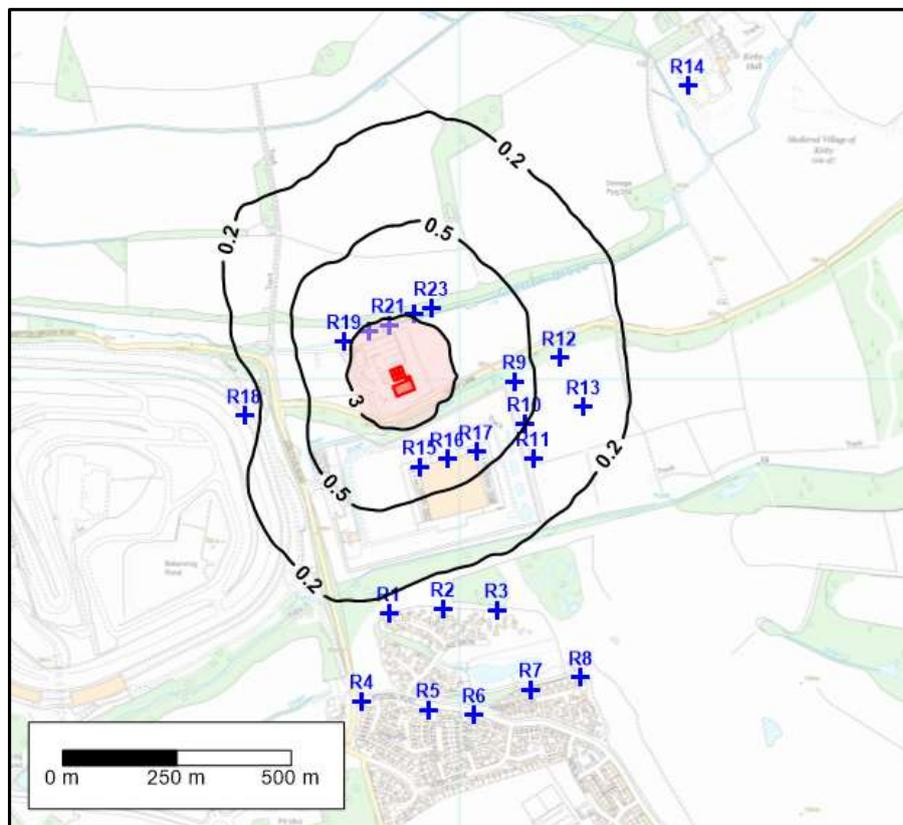
Figure 5.2 ADMS 5.2 Predicted 98<sup>th</sup> Percentile of Hourly Average Odour Concentration, 2016 Meteorological Data ( $OU_e m^{-3}$ )
