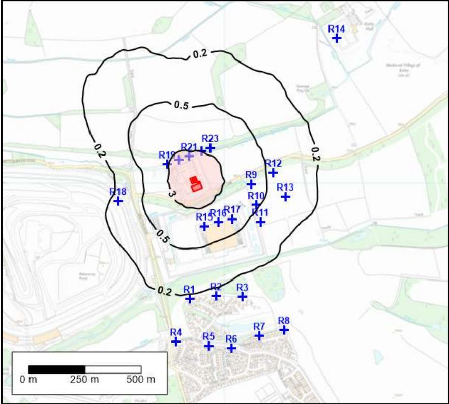
**Figure 5.5 ADMS 5.2 Predicted 98<sup>th</sup> Percentile of Hourly Average Odour Concentration, 2019 Meteorological Data (OU<sub>e</sub> m<sup>-3</sup>)**
